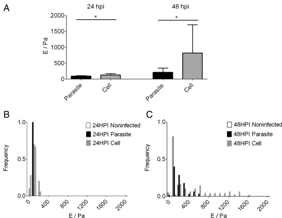
Figure 3. (A) Results of nanoindentation comparing results on infected cells measured directly over the parasite location (EEF) and over the main body of the cell. Starred pairs were significantly different ( $P < 0.05$ ). (B and C) histograms illustrating the distribution of values obtained by nanoindentation measurements on cells 24 (B) and 48 (C) hpi.
